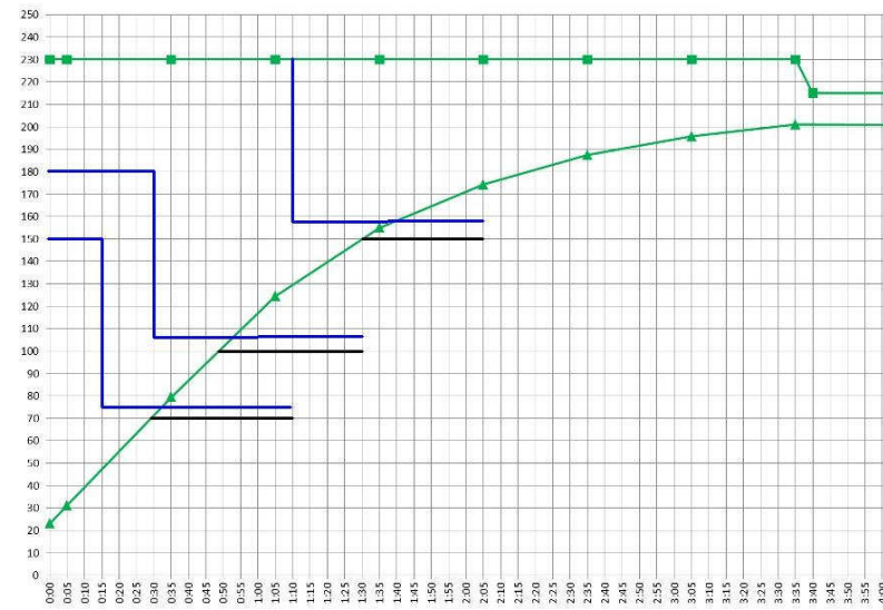
Fig. 26 Heating progress for a 230 °C set point of the heating box for the metallic recipient.
