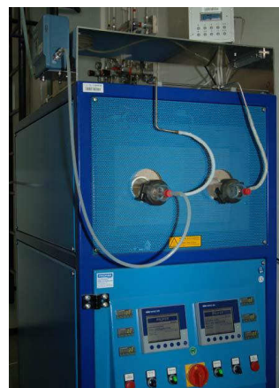
Fig. 28 The set-up of long term annealing experiments.
