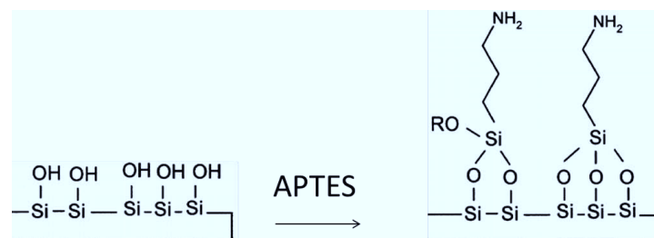
Fig. 13 Atomic layer deposition (ALD) of the amino-propyl-siloxane layer [84]
